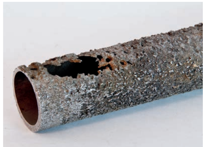
Figure 6.7. Uniform corrosion on the outside of a steam tube exposed to sulphuric acid.
