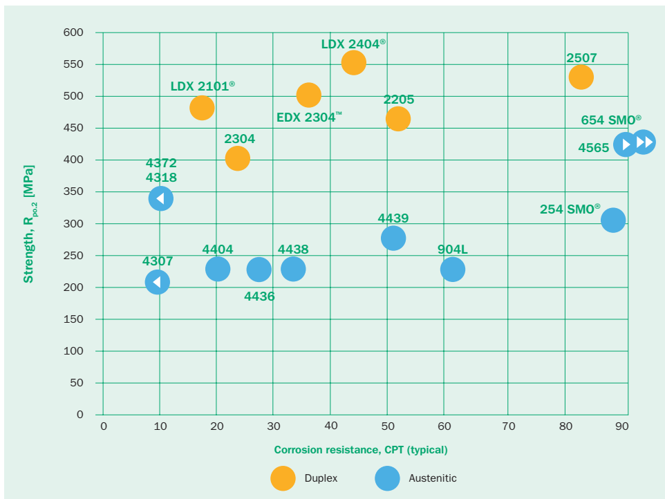
Figure 9:16. Proof strength (min. values for hot rolled coil acc. to EN 10088-2) for some austenitic and duplex grades in relation to their corrosion resistance (CPT acc. to ASTM G150). Grade EDX 2304™ has a balanced chemical composition to obtain optimal corrosion resistance and strength, but it still correspond to EN 1.4362 and UNS S32304.
