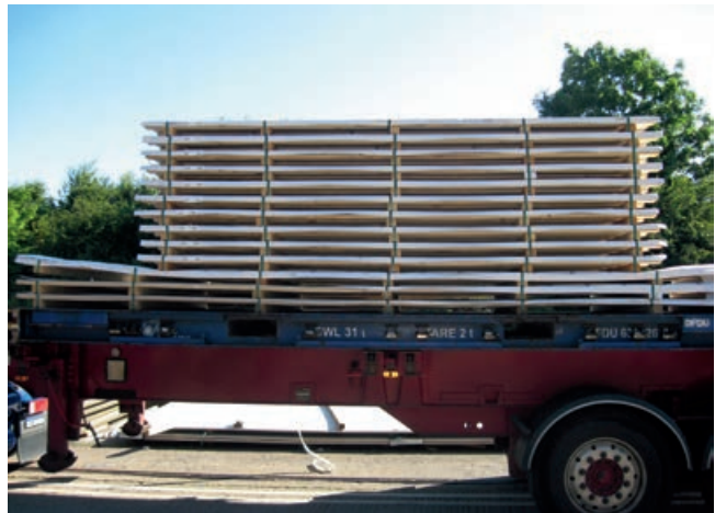
Figure 12:3. Example of careless loading. The bottom plates have lost their flatness.
