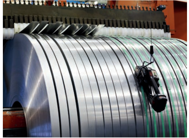
Figure 4:14. A coil that has been slitted into several narrow coils.
