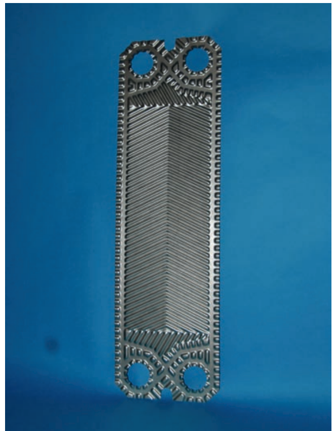
Figure 9:12. The formability of e.g. grade 654 SMO ® is excellent.
