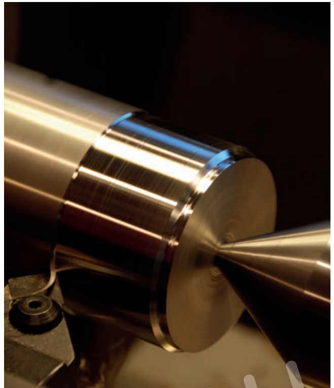
Figure 9:6. Duplex grade LDX 2101 ® shows excellent machinability.
